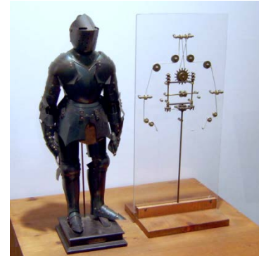
Figure 1.2: Model of a robot knight based on drawings by Leonardo da Vinchi.
