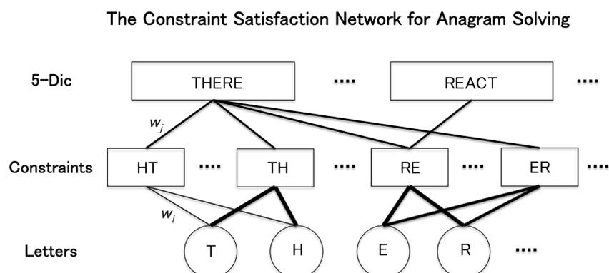
**Figure 1. A 3-layer constraint satisfaction network. The bottom layer consists of 26 letters in English alphabet. The weights ( $w_i$ ,  $w_j$ ) represent the constraints for the combinations of the letters. The feed-forward network represents the anagram solver's constraint satisfaction network.**
