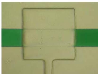
**Figure 5.** A fully closed pneumatic valve (300x300  $\mu\text{m}$  square) over a 100  $\mu\text{m}$  channel, effectively blocking the channel filled with green dye.
