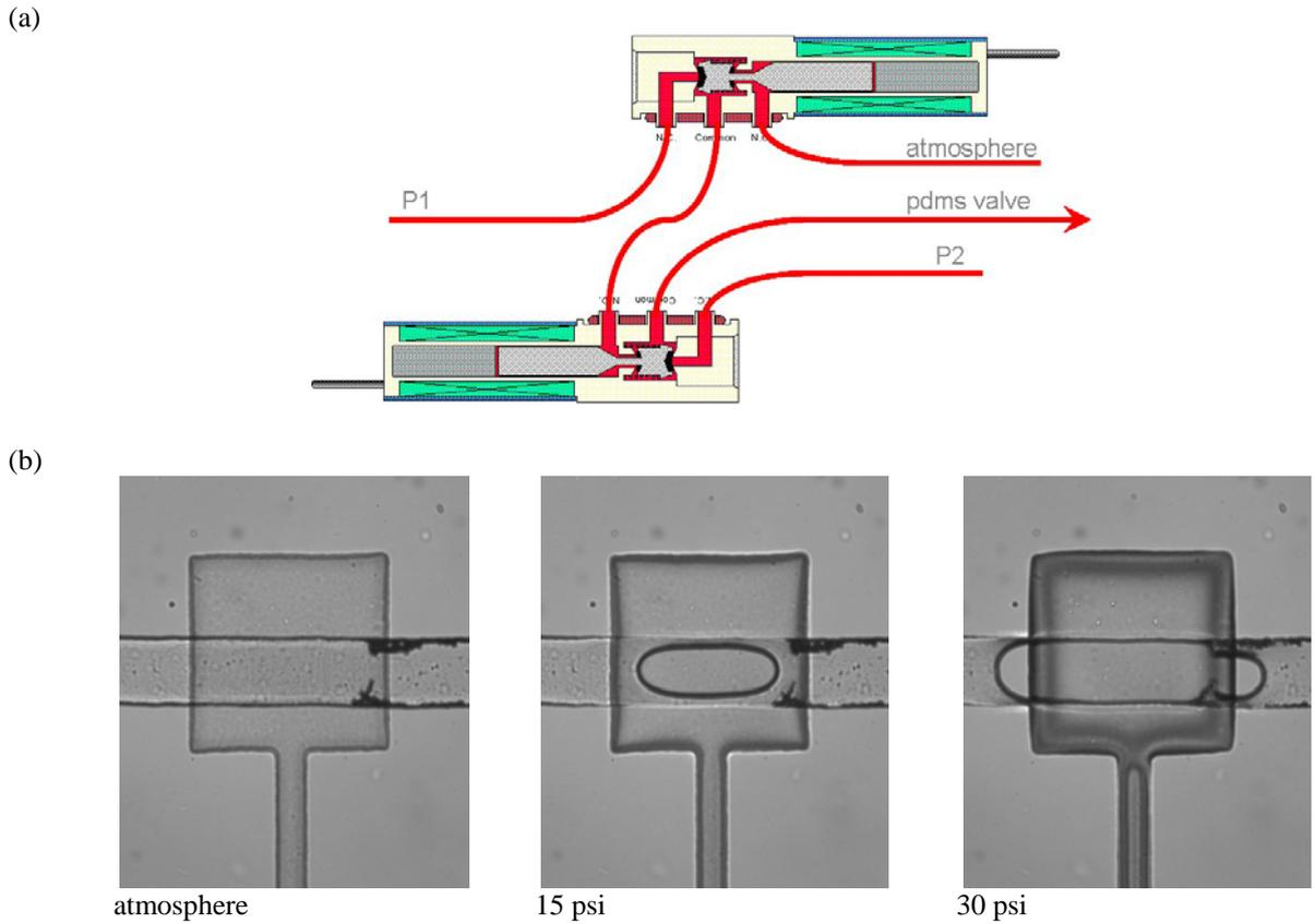
**Figure 8.** (a) By putting 2 bi-stable solenoid valves in series it is possible to apply 3 different pressures to the PDMS valves, where  $P_i$  is the pressure. (b) The pneumatic PDMS valve (300x300 μm square) over a 100 μm channel at atmosphere, 15 and 30 psi. As can be seen, at 15 psi the valve is not completely closed, allowing for a decreased flow, but retaining the beads.
