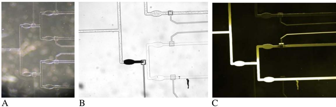
**Figure 7.** (a) the reactor layout in PDMS, containing 6 valves after each of the 6 reactors. (b) a reactor being filled with beads. Notice that only where the valve is partially closed beads are trapped. (c) a fluorescence image of a flow path with Rhodamine 6G through the microsystem. By completely closing the valve, the flow direction can be regulated.
