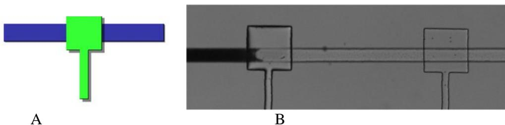
**Figure 6.** (a) a schematic representation of a valve. The dark gray channel is the solution flow channel, while the light gray channel is the pneumatic valve over the flow channel separated by a 40  $\mu\text{m}$  membrane. (b) 5.6  $\mu\text{m}$  beads (on the left side of the valve) were collected before a partially closed valve. The flow channel is 100  $\mu\text{m}$  and the valve pad is 300x300  $\mu\text{m}$ .
