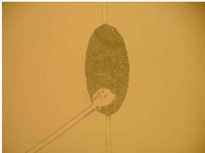
**Figure 4.** 5.6  $\mu\text{m}$  beads in a reactor were the vertical in- and output channels (50  $\mu\text{m}$  wide, 3  $\mu\text{m}$  deep) function as bead barriers, while the diagonal bead delivery channel (100  $\mu\text{m}$  wide, 10  $\mu\text{m}$  deep) has the same depth as the reactor.
