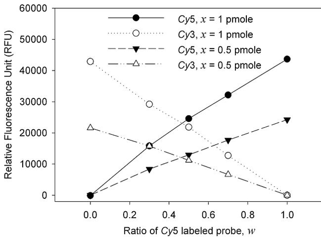
**Fig. 3.** Weight encoding verification. The resulting relative fluorescence unit (RFU) representing the multiplication results of single-input and weight pairs increased linearly with the input level,  $x$ , and the mixing ratio of the corresponding probe. The black solid symbols denote the signal from Cy5, i.e.  $xw$ , and the white symbols denote the signal from Cy3, i.e.  $x(1 - w)$ .
