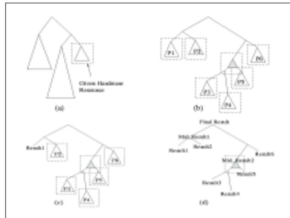
Fig. 6. This shows context switching procedure. Dashed square box represents given hardware resource. In context switching, the tree is divided into subtrees whose size is representable on hardware.
