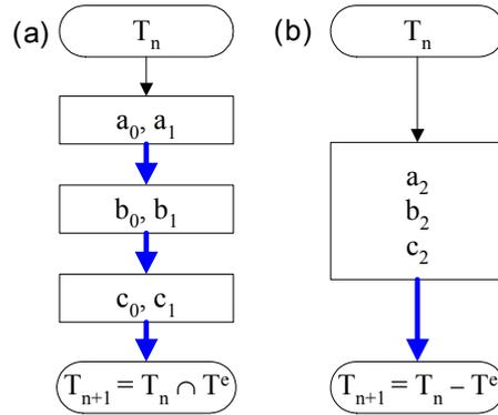
**Fig. 2.** Modified version of the learning process, which uses only positive selection for an example  $\langle a_1, b_1, c_1 \rangle$ . (a) is for a positive example, and (b) is for a negative example
